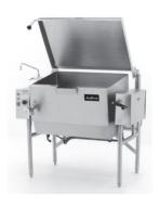
AccuTemp Edge Series™ Tilting Skillet, Gas, 40 gallon capacity, thermostatically controlled, self-locking worm gear & tilt mechanism, heavy duty actuator-assisted cover with condensate drip shield & cover vent, includes optional direct spark ignition combination gas control, 304 stainless steel & clad pan body construction, open 1-5/8″ tubular leg stand, 120,000 BTU, 120v/60/1-ph, UL, NSF
